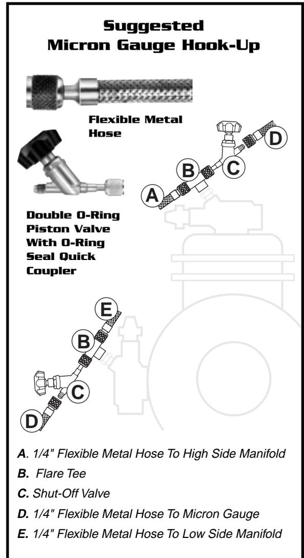
The most accurate reading is obtained at the compressor using both the high and low sides. At this point, we need some additional connections for our electronic gauge, and some provisions for charging must be considered.
