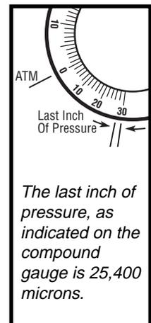
*The last inch of pressure, as indicated on the compound gauge is 25,400 microns.*
