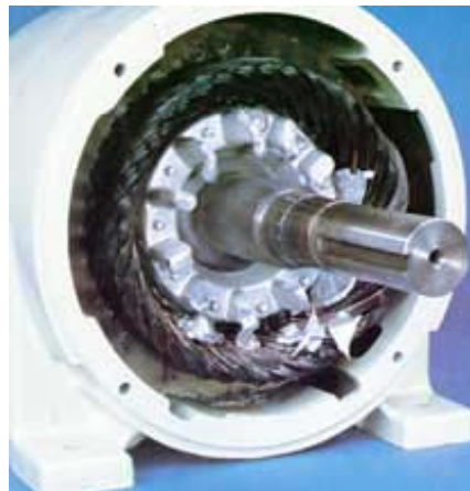
11. Damage Caused by Locked Rotor
