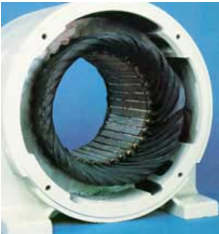
10. Winding Damage Due to Overload
