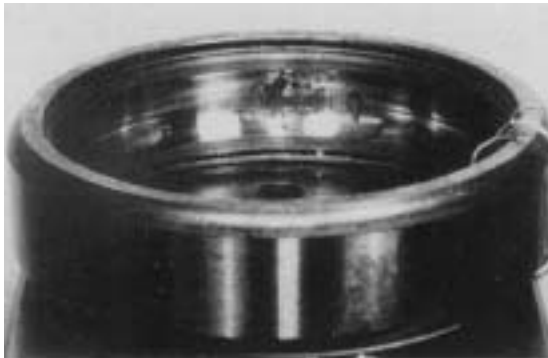
Damaged caused by water intrusion
