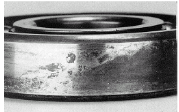
Fretting corrosion caused by loss of fit and vibration
