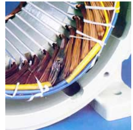
12. Winding Damaged by Voltage Surge
