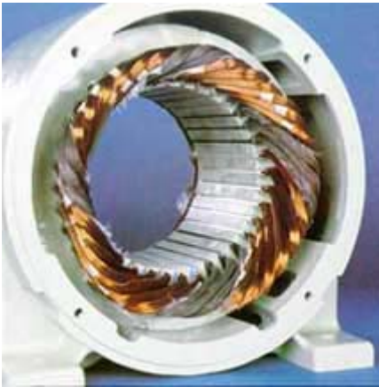
2. Winding Single-Phase ( \Delta - connected)
