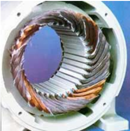
1. Winding Single-Phase (Y - Connected)
