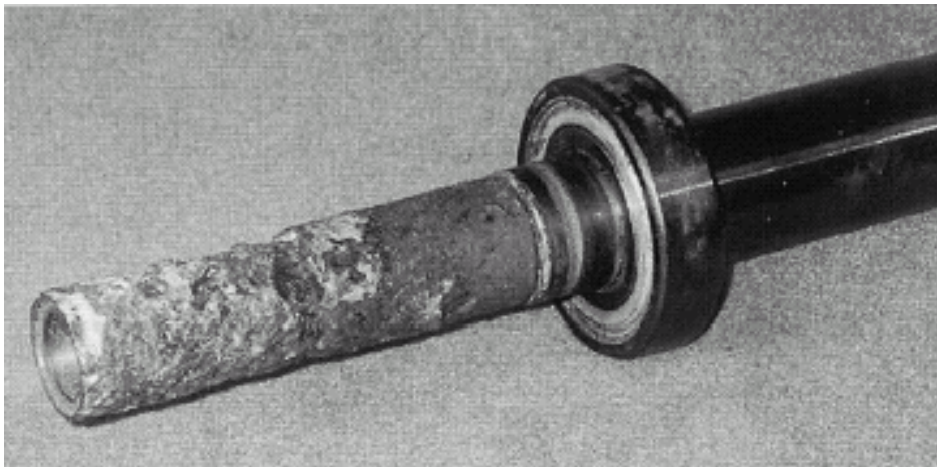
Extreme corrosion, wear and cracking on a pump shaft
