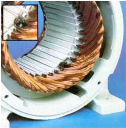
6. Winding Grounded at Edge of Slot
