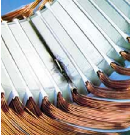
7. Winding Grounded in Slot
