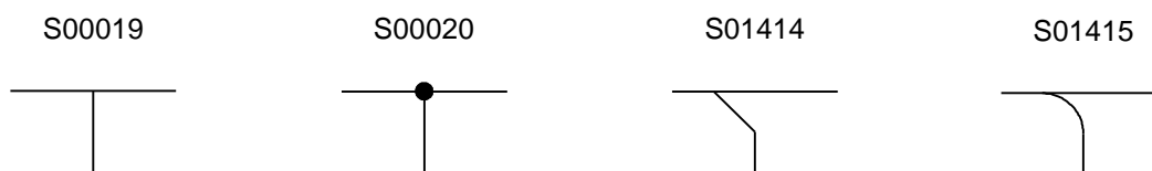
Figure 18 – Symbols representing joining of connecting lines
