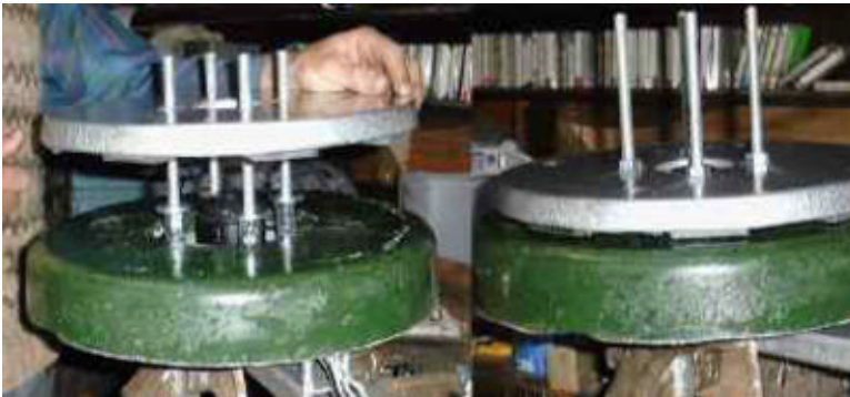
Fitting the front magnet rotor
