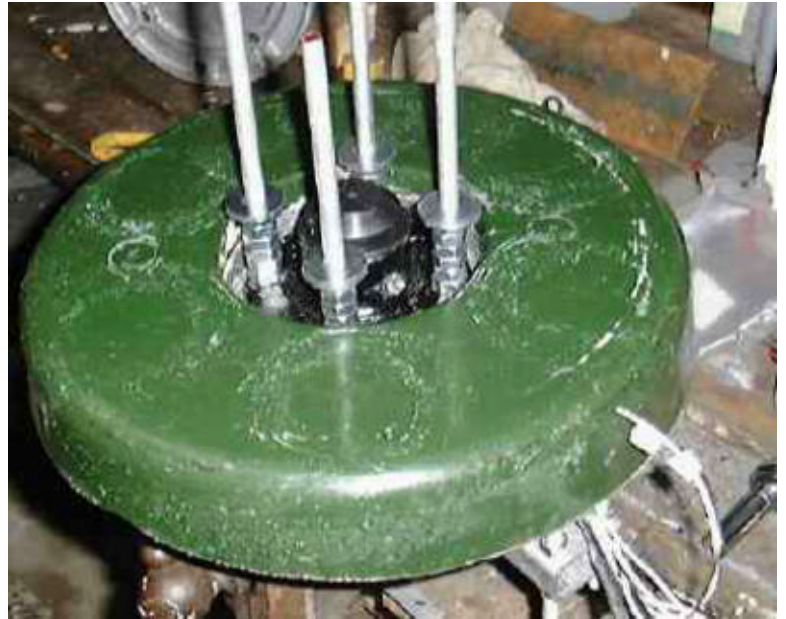
Fitting the stator
