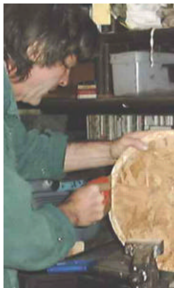
Sawing flat faces on the inner mould
