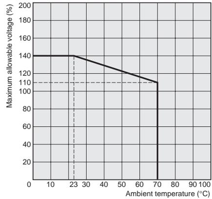
**Note:** The maximum allowable voltage is the maximum possible value of the voltage that can be applied to the relay coil.
