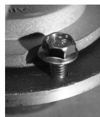
A. Place flange cutouts over 5/16–18 NC bolts installed in mount or accessory.
