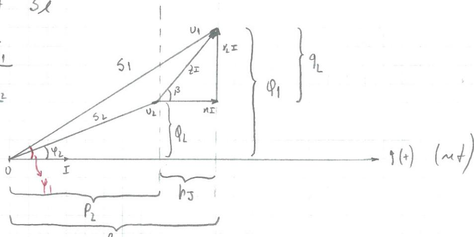
$$① \Rightarrow 3 \cdot U_1 \angle \varphi_1 \cdot I \angle \varphi_1 = 3 U_2 \angle \varphi_2 \cdot I \angle \varphi_2 + 3 \bar{z} I^2$$
