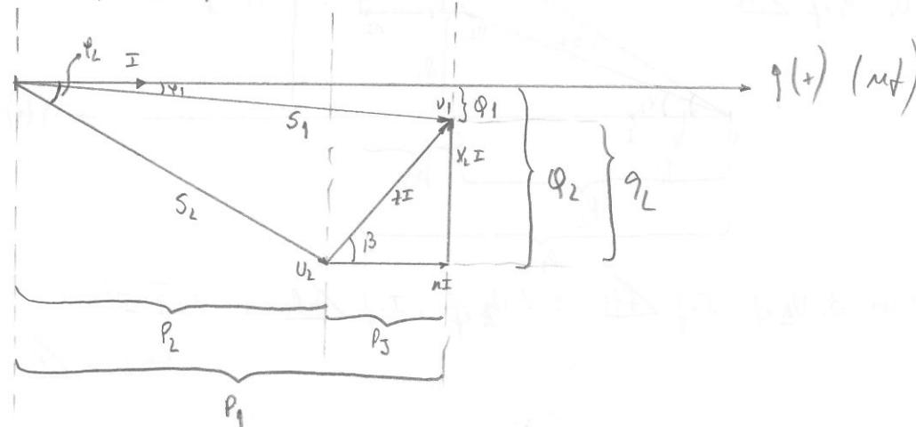
$$\textcircled{2} \quad 3 \cdot U_{1,\text{ef}} \cdot I_{1f} \angle -\varphi_1 = 3 U_{2,\text{ef}} \cdot I_{1f} \angle -\varphi_2 + 3 Z \cdot I^2$$
