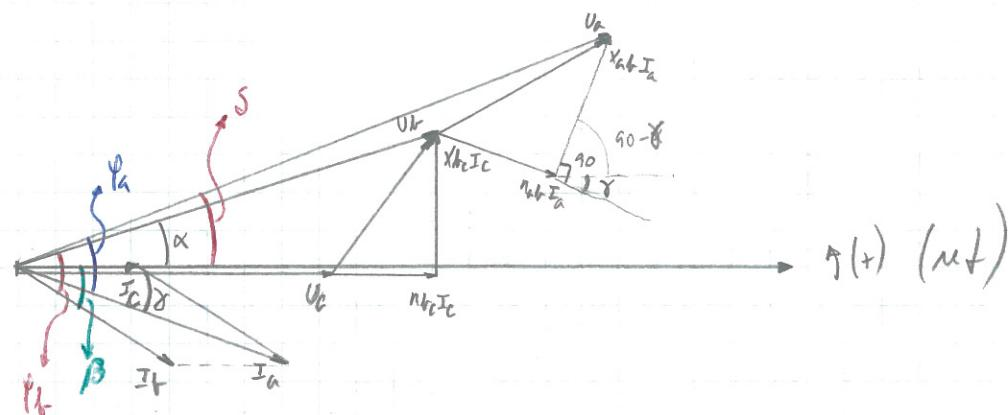
$$\bar{U}_b = \bar{U}_a + (n_b I_b + j X_b I_c) \bar{I}_c$$
