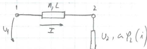
$$\bar{U}_1 = \bar{U}_2 + (n + jx_L) \bar{I} = \bar{U}_2 + z \bar{I} \Rightarrow \bar{U}_1 - \bar{U}_2 = z \bar{I}$$
