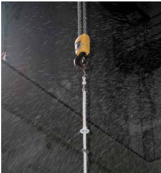
Fig. 5.7.1.3 Withstand voltage test under sprinkling
