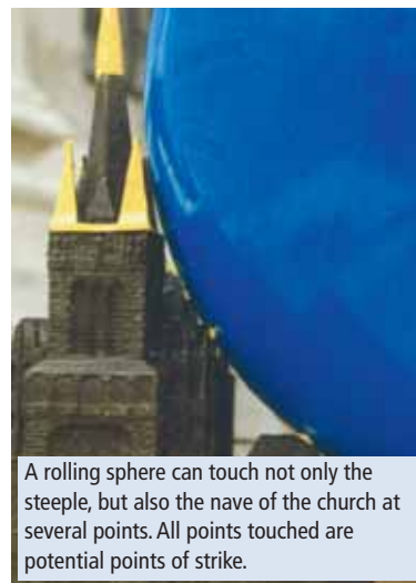
Fig. 5.1.1.2 Model of a rolling sphere Ref: Prof. Dr. A. Kern, Aachen
