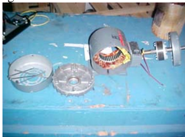
Figure 12: Disassembled Test Motor
