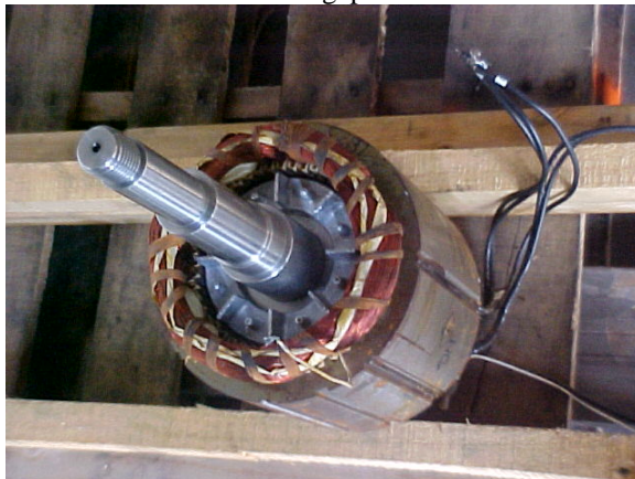
Figure 15: Virtual Motor with Spacers to Hold Airgap
